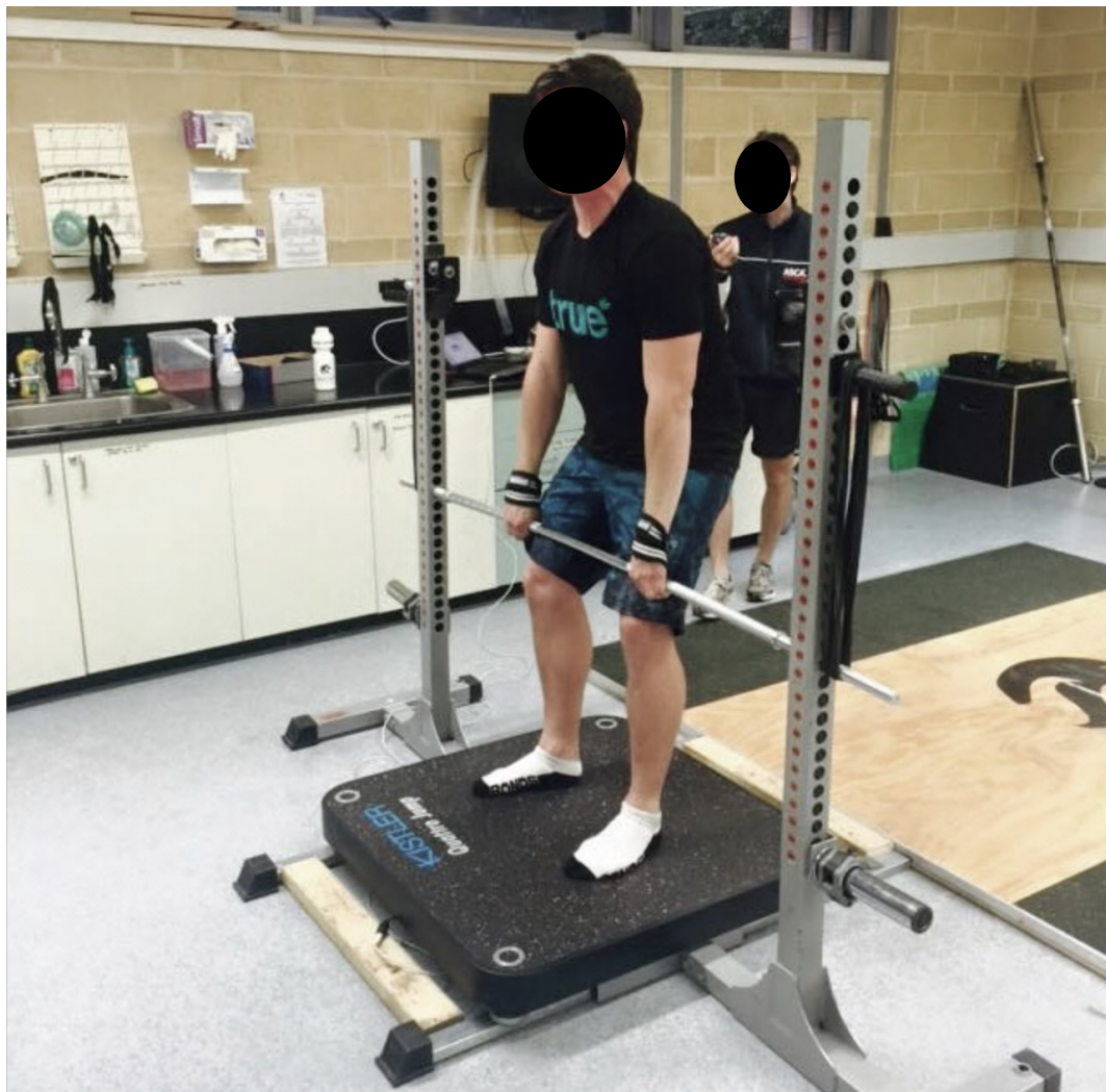
Figure 7.1. Isometric mid-thigh pull using a customised power rack and force platform.
